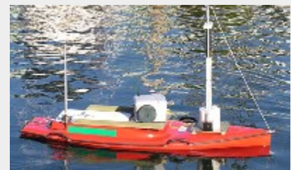
Roboboat - Researchers from USC are working with a roboticist to study the effects of red tide on harbor waters using a radio-controlled boat.
