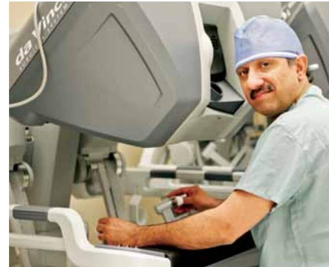
Inderbir Gill, M.D., M.Ch., sits at the da Vinci surgical system console, where every movement of his hands is mimicked by robotic arms on the patient cart just a few feet away.
