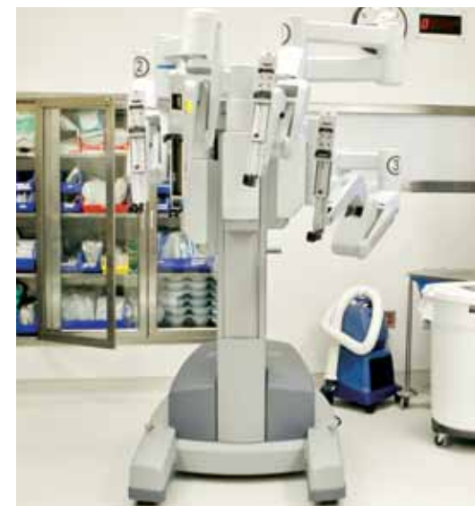
Top: The four interactive robotic arms of the da Vinci surgical system hold and reposition surgical instruments and a camera during surgery. Bottom, left: The console where the surgeon works, using hand controls and foot pedals to remotely manipulate the robot's arms with very high precision. Middle: When looking through the two lenses, the console provides a highly magnified 3D image of the body's interior. Right: A view of the entire patient cart with robotic arms.
