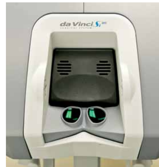
Top: The four interactive robotic arms of the da Vinci surgical system hold and reposition surgical instruments and a camera during surgery. Bottom, left: The console where the surgeon works, using hand controls and foot pedals to remotely manipulate the robot's arms with very high precision. Middle: When looking through the two lenses, the console provides a highly magnified 3D image of the body's interior. Right: A view of the entire patient cart with robotic arms.
