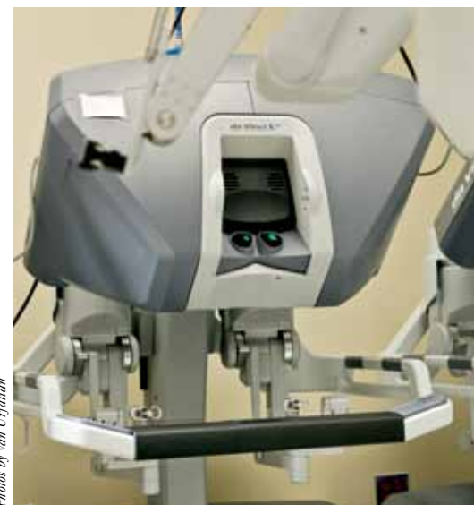
Top: The four interactive robotic arms of the da Vinci surgical system hold and reposition surgical instruments and a camera during surgery. Bottom, left: The console where the surgeon works, using hand controls and foot pedals to remotely manipulate the robot's arms with very high precision. Middle: When looking through the two lenses, the console provides a highly magnified 3D image of the body's interior. Right: A view of the entire patient cart with robotic arms.
